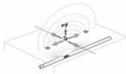
Figure 27: Poles and Equator of a Sonde
